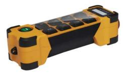
This system is offered in a 6 pushbutton, dual speed controller with two auxiliary buttons. It has a "start" button and an Emergency Stop. A great feature of this controller is that the auxiliary buttons can be used to operate dual hoists (independent of one another) or simultaneously by pushing button 1 & 2 at the same time.
