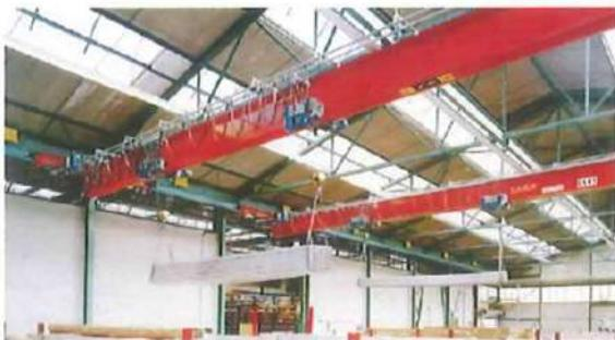
The single/double girder under-slung crane can be directly installed on the roof structure of existing plant without additional crane rail, which can make all the place being the working area. Moreover, it can be only used in part of plant area according to request. The traveling range of trolley can exceed the crane span through using the side cantilever. The max. Lifting capacity is 5 ton.
