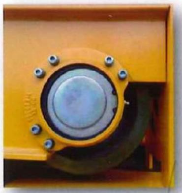
wheel with self-aligning bearing
