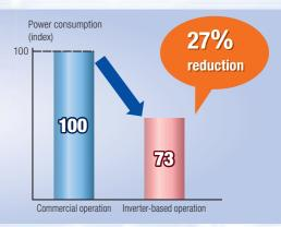
Reduction in power consumption that is achieved when a 3t inverter hoist is operated with cycles of 5 times per hour with the hoist installed on a crane with a hoisting lift of 6m, a span of 12m and a 50m runway.
