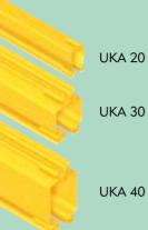
Load capacity from 125 to 2000 kg according to profile type. The system is based on a special hollow profile, which is manufactured in cold formed metal sheet in order to obtain an extremely smooth and regular surface. The closed structure of the profile makes it possible to keep the inside of the running surface clean.
