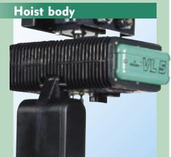
Made with moulded injected aluminium, making the hoist lighter, the fins on the motor section provide good thermal exchange. The chassis is painted with one Coat of 2-component epoxy paint with 80 microns that is highly resistant to corrosive agents.
