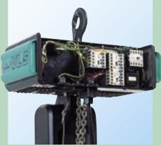
Quite large, built into the piece of equipment, it contains all of the component (plate, connectors, transformer, etc.) and is easy to access for maintenance purposes, IP55 protection.
